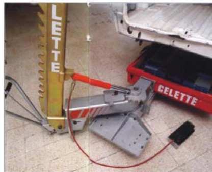
Beams pivots for multi-angle pulling
