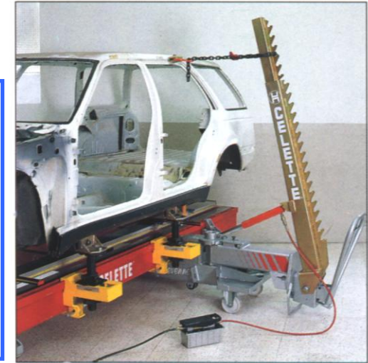
High level pulls using vertical extension 9128.503
