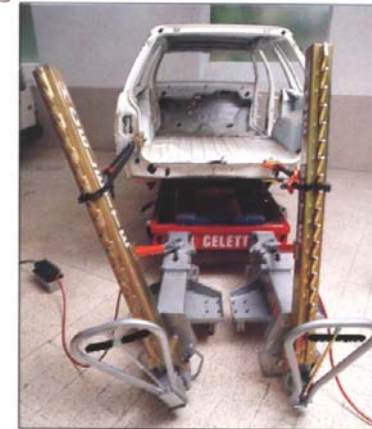
Two pullers can be fitted side by side
