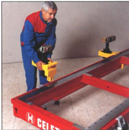
Sill clamps are very easy to fit
